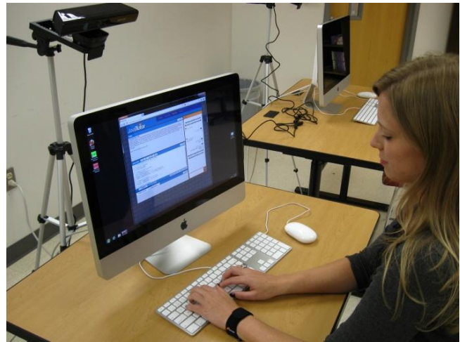
Figure 1. Student workstation with depth camera, skin conductance bracelet, and computer with webcam
